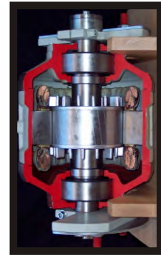
A look inside the LR Series' vibratory motor
