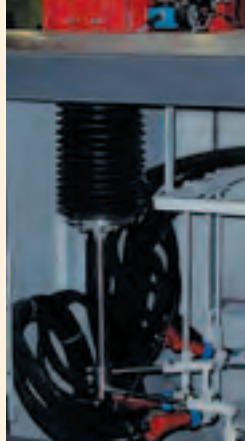
Devices for vertical and horizontal nozzle movements
