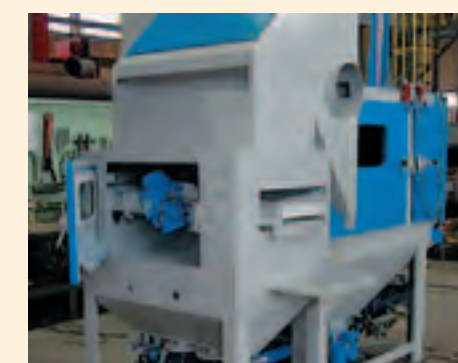
Processing system for blasting media.
