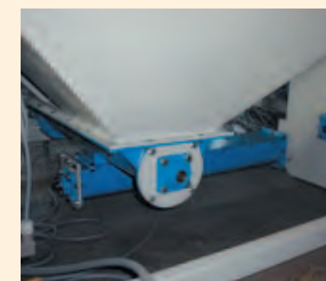
Blasting media screw and elevator
